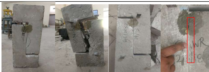
Fig.4. Failure Pattern for unreinforced and reinforced across shear plane
