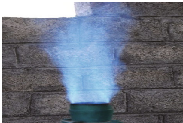
Fig. 3 Blue flame from the burner of the gasifier
