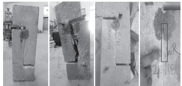
Fig. 4 Failure pattern for unreinforced and reinforced across shear plane
