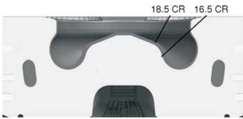
Figure 2. Piston bowl geometry modification to achieve 16.5 CR
