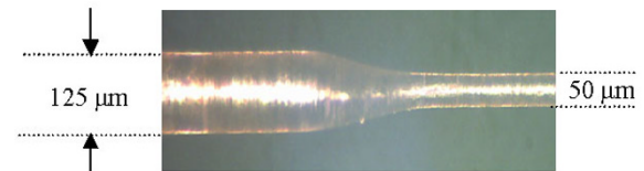
Fig. 2 Unetched and etched parts of the fiber.
