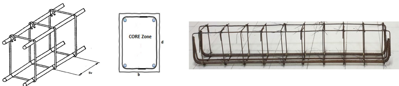
Fig. 2 Reinforcement cage and cross section with conventional stirrups
