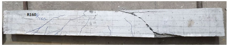
(a) R160 Beam Crack pattern at Ultimate –Failed in Shear
