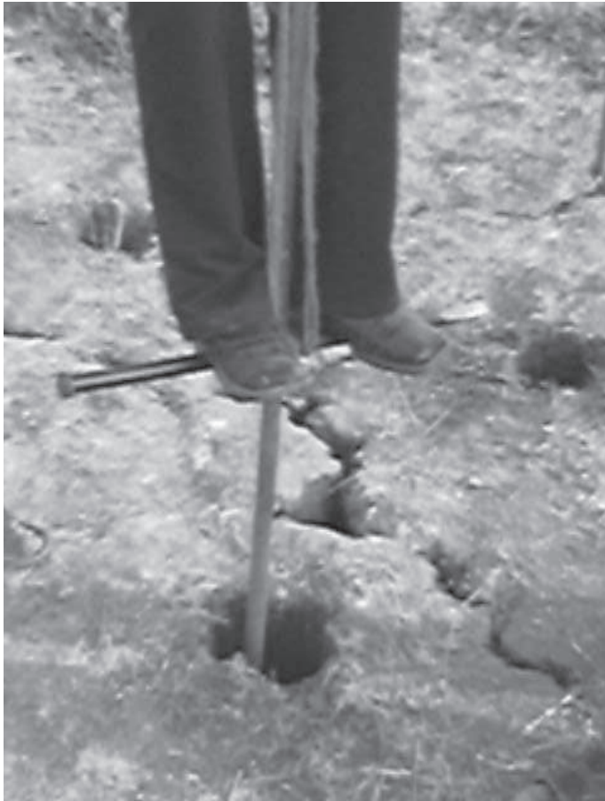
Figure 3. Picture depicting auger boring at test site for lime slurry treatment.
