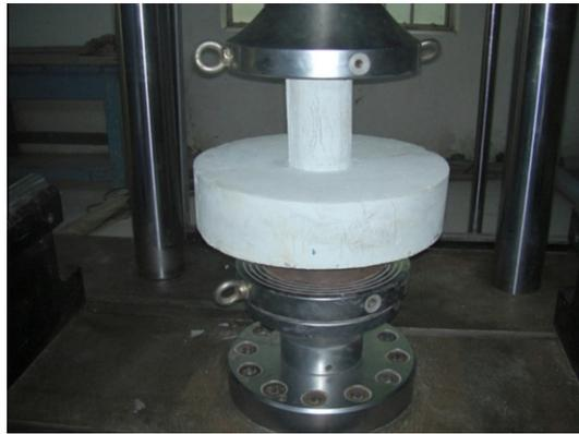
**Fig. 7.** Photograph of slab column specimen in the testing machine.
