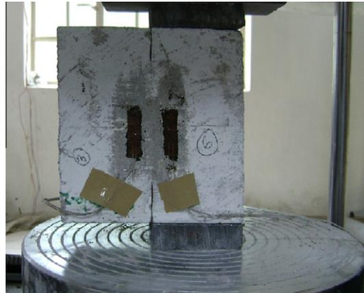
Fig. 2. Photograph of double edge notched specimen in the testing machine.
