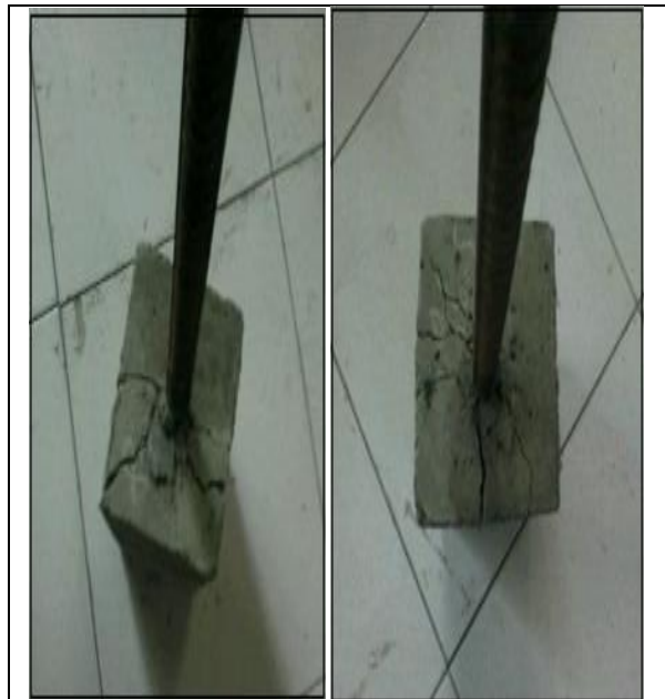
Figure 6: Failure pattern of specimens
