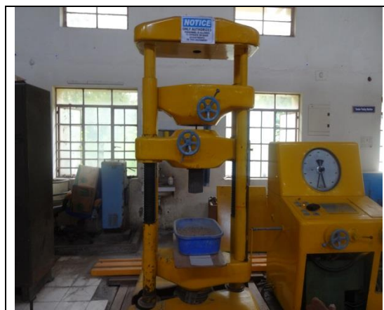
Figure 3: Pull out test setup
