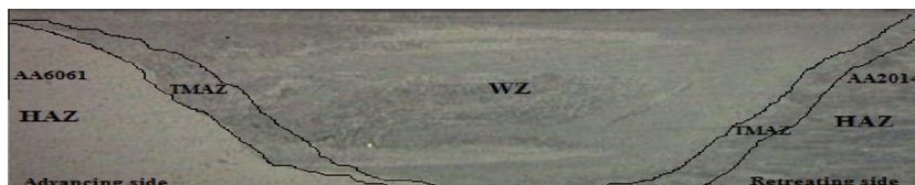
Fig. 12. Cross section of the welded blank with different weld zones.
