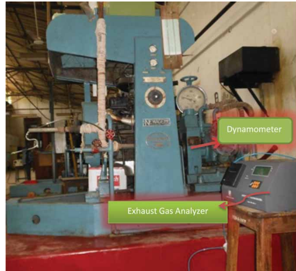
Figure 1. The pictorial representation of the experimental set-up.
