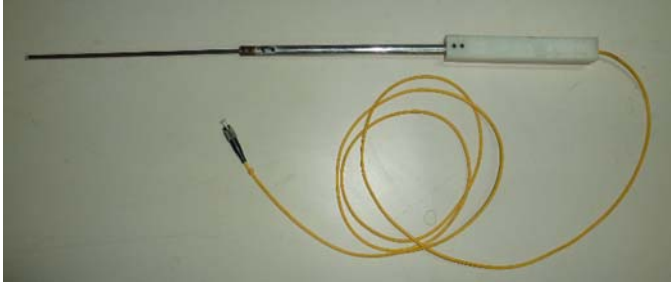
Fig. 1. Photograph of FBG sensor probe
