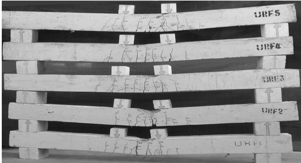
Figure 8 : GFRSCC beams showing crack pattern
