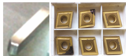
Fig. 3—HSS tool and carbide inserts
