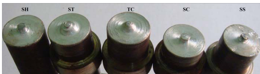
Fig. 1 Photographs of different tool pin profiles
