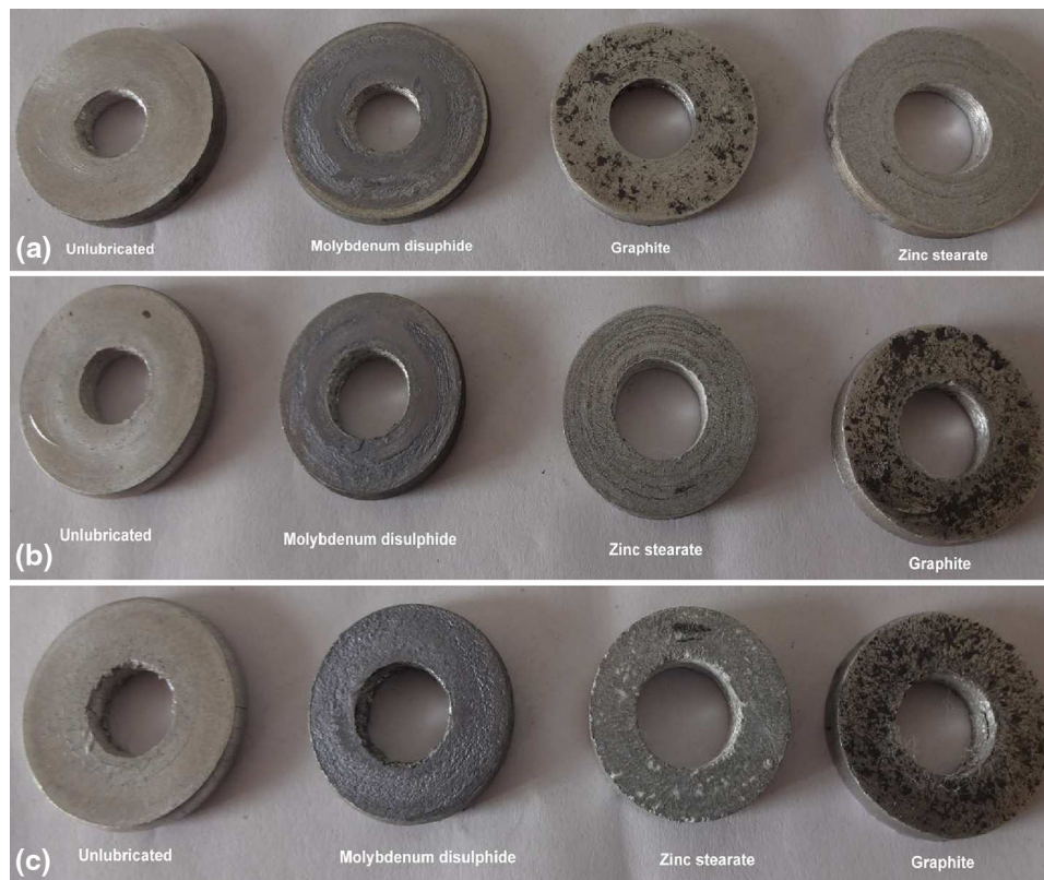
Fig. 8 Photographs of deformed ring specimens under different lubricating conditions to height reduction of 45% for initial relative densities of (a) 0.9 (b) 0.85 and (c) 0.75
