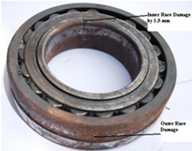
Fig. 2 Inner race and cage with defects
