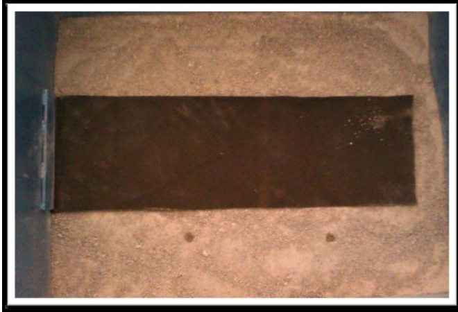
Figure 4 Embedment of Geotextile into pullout box
