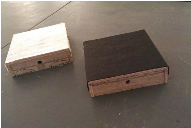
Figure 2 Geotextiles nailed to wooden box
