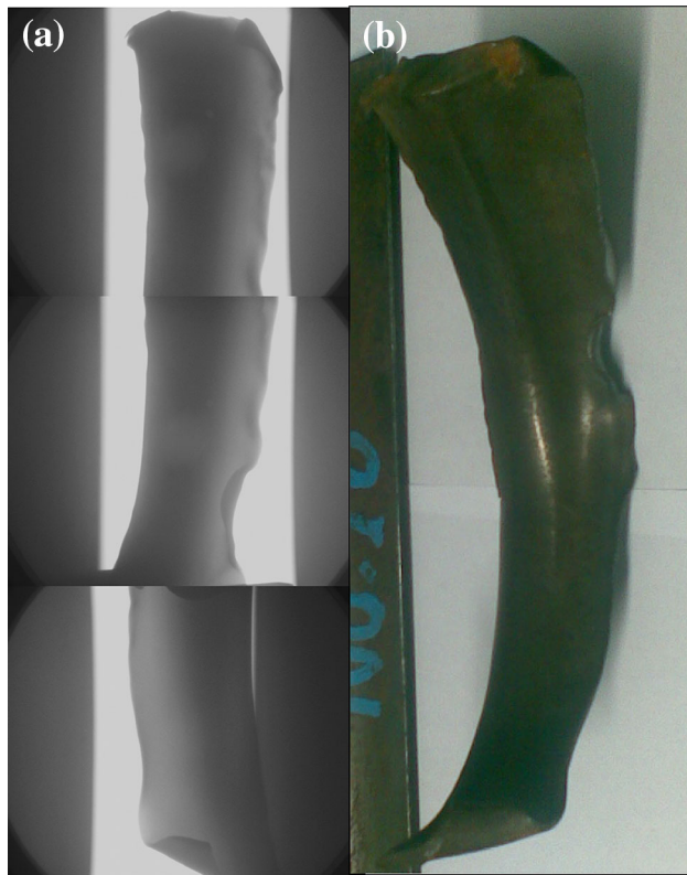
Fig. 3 (a) X-ray radiography images of the failed blade, 80 kV \times 5 mA (b) photograph of as-received failed blade
