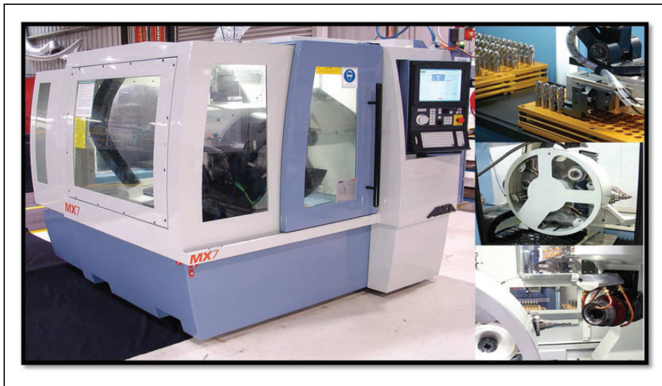
Figure 5. ANCA MX7 CNC tool end cutter machine.
