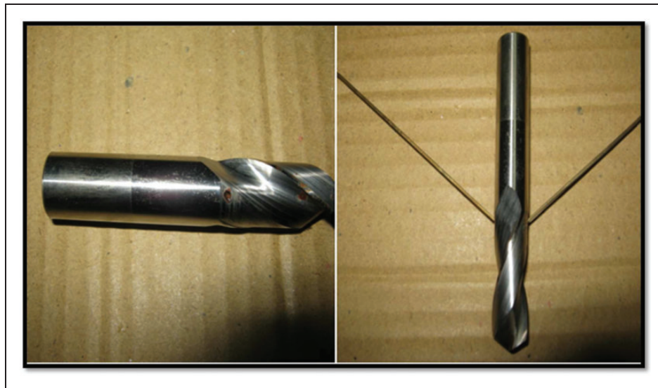
Figure 6. Drilled tool bits of side holes.
