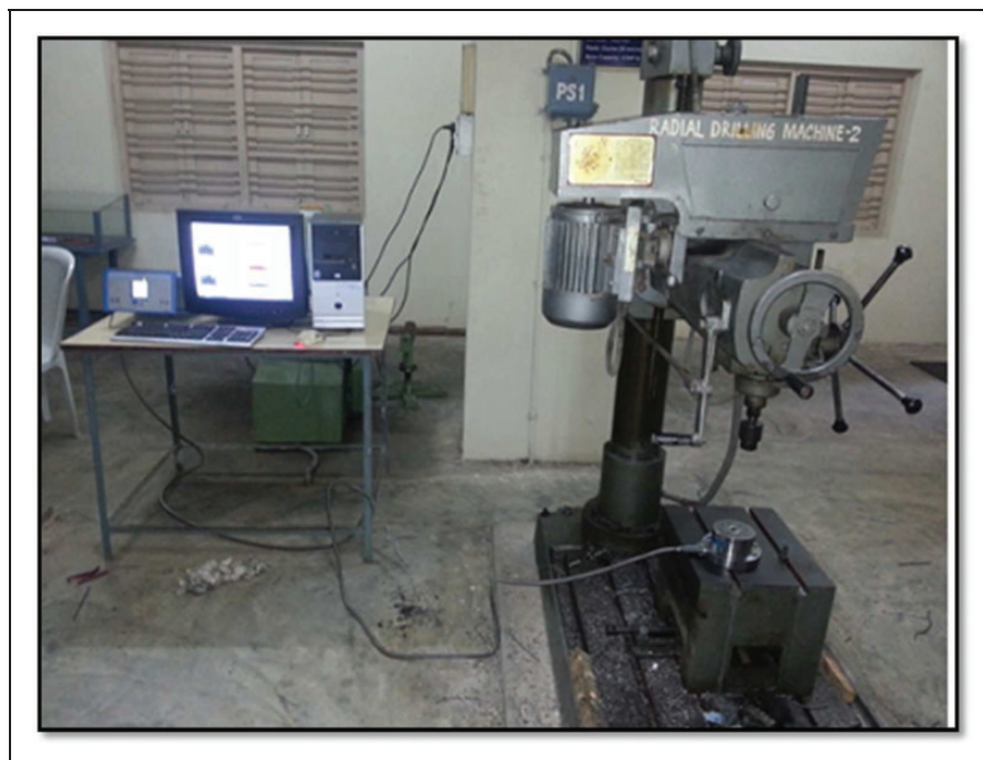
Figure 8. Experimental setup of dynamometer mounting on radial drilling machine.
