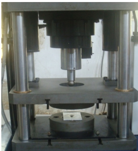
Fig. 2 Assembly of dies and punch used in LDH test
