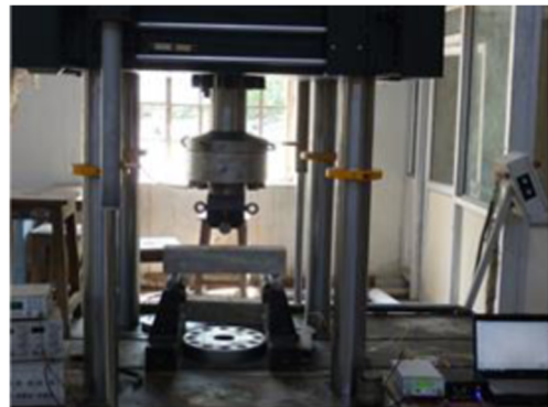
Fig. 8 Photograph of the Experimental Setup for the Three point bend test of Concrete Beam on 1000KN Digital controlled UTM at Materials Laboratory, Civil Engineering Laboratory NIT, Warangal
