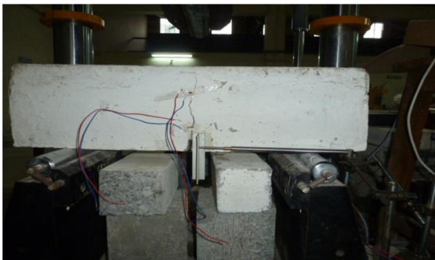
Fig. 7 Photograph showing a LVDT mounted close to the concrete beam at the prenotch
