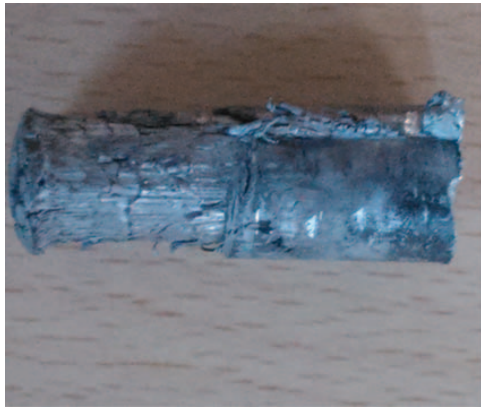
15 Thixoextruded specimen cracked due to fluid segregation
