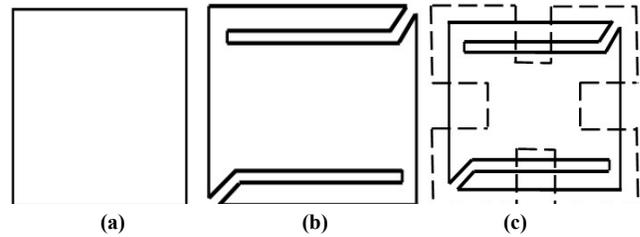
Fig. 2. Design iterations-(a) basic patch (b) L-shaped spur lines without DGS (c) Spur lines with Hilbert fractal DGS
