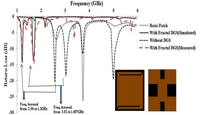
Fig. 3. Simulated and Measured Return loss of propose
