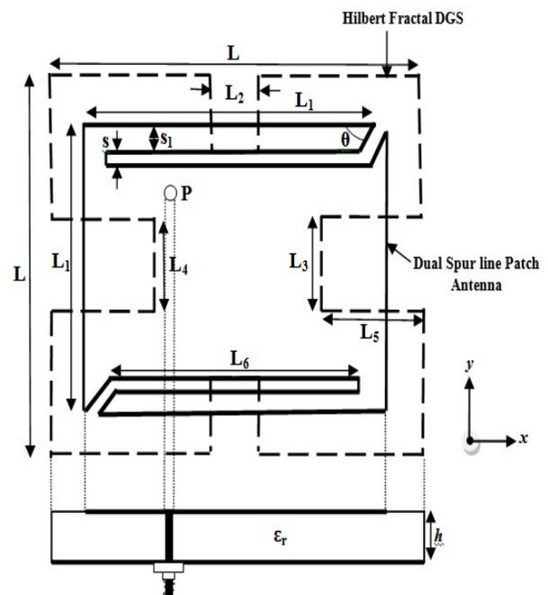
Fig. 1. Geometry of the Proposed Antenna (All dimensions in mm)
