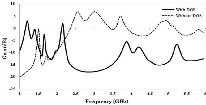
Fig. 4. Gain versus frequency response for proposed antenna with and without fractal DGS
