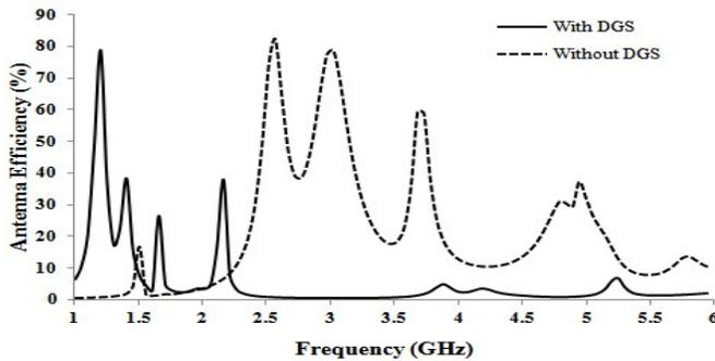
Fig. 5. Measured Antenna efficiency for proposed antenna with and without fractal DGS
