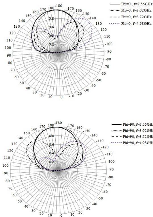
Fig. 6. E-plane Radiation patterns for  $\phi=0^\circ$  and  $\phi=90^\circ$  at resonant frequencies of 2.56, 3.02, 3.72 and 4.98 GHz ( $y-z$  plane). (Without DGS)
