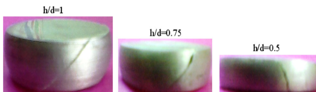
Fig. 1 Billets of different aspect ratios ( h/d ) after upsetting to the fracture limit
