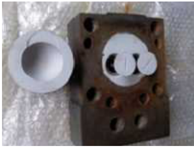
Fig. 1. LZ coated piston, valves and cylinder head
