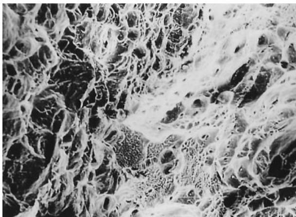
Fig. 3. Scanning electron fractograph of a broken test specimen with a relatively high fracture toughness (95–102 MPa√m) (Magnification x150)
