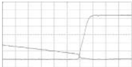
Fig. 12(d): BPS left-leg ZVS turn-off transient (Voltage: 50 V/div., Current: 1 A/div., Time: 200 nsecs./div.)
