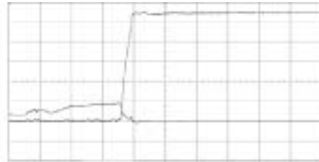
Fig. 13(d): FPS left-leg ZVS turn-off transient (Voltage: 50 V/div., Current: 1 A/div., Time: 200 nsecs./div.)
