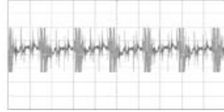
Fig. 15(d): Experimental output voltage waveform (Voltage: 0.5 V/div., Time: 5 μsecs./div.)
