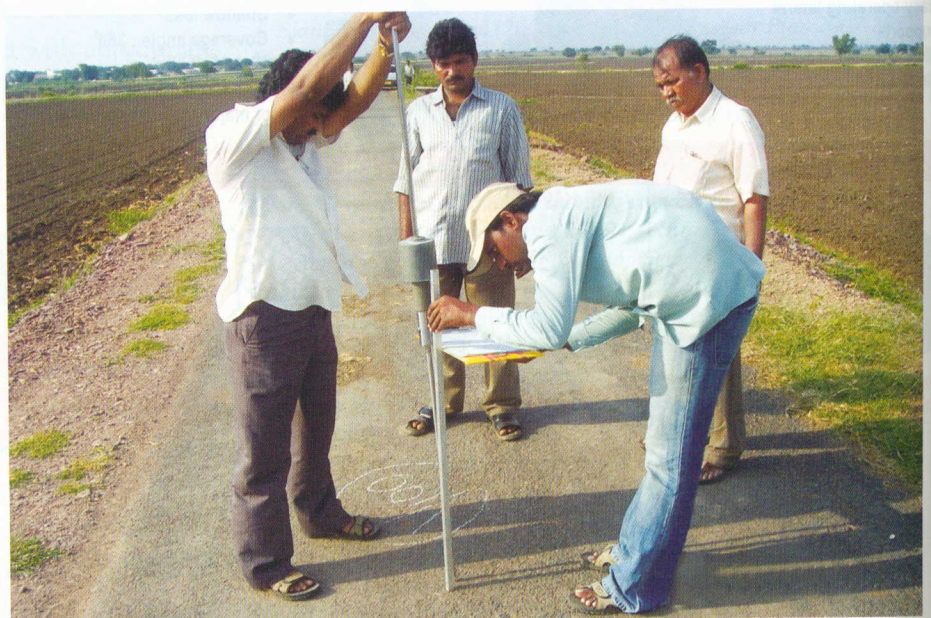
Fig 1: Measuring The Properties Of Pavement Layers Through Dynamic Cone Penetration (DCP) Equipment
