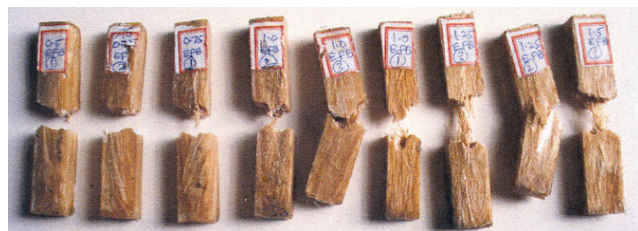
Fig. 7—Photograph showing fractured sample specimens of banana-ECF composites in impact testing
