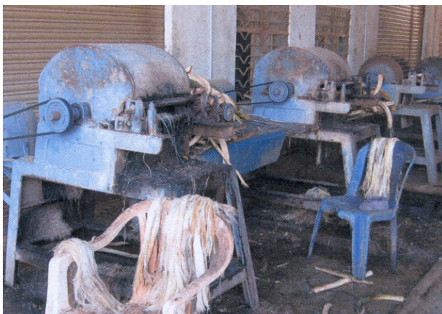
Fig. 2—Decorticating machine used for extraction of fibre
