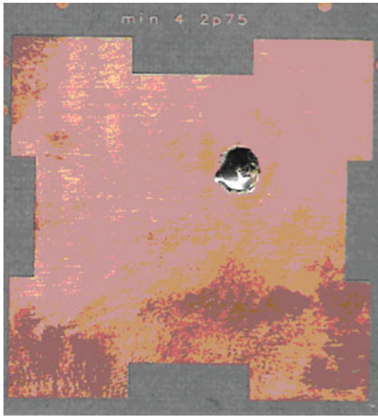
Figure 8. Photograph of fabricated fractal boundary CP antennas with indentation depth factor (0.3,0.2) and indentation angle 90^\circ . [Color figure can be viewed in the online issue, which is available at www.interscience.wiley.com .]
