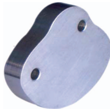
Figure 6. Plate cam manufactured on CNC machine.
