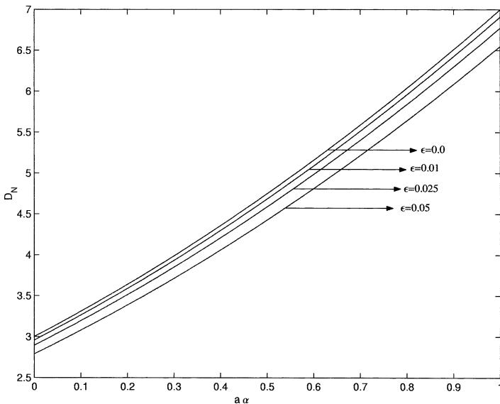
**Figure 2.** Variation of drag coefficient ( $D_N$ ) with  $a\alpha$  (oblate spheroid).
