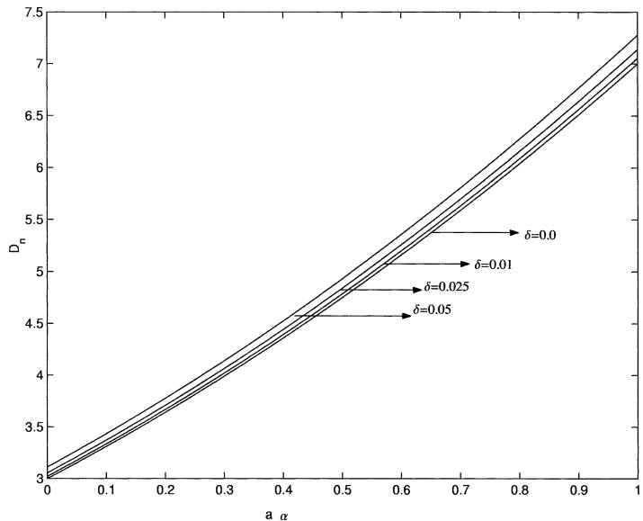
**Figure 1.** Variation of drag coefficient ( $D_N$ ) with  $a\alpha$  (approximate sphere with  $\beta_2 = \beta_4 = \delta$ ).
