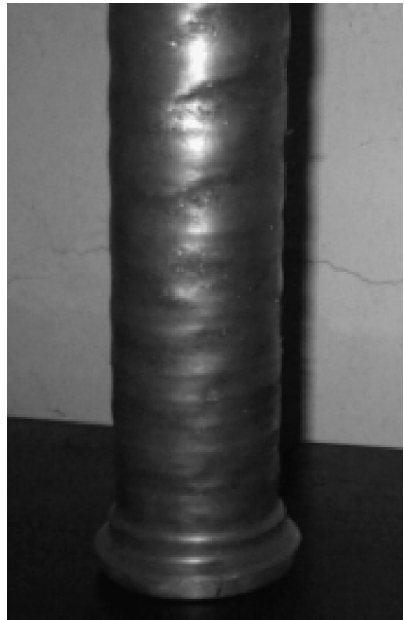
Fig. 1 – A flow-formed tube with wave-like surface-type quality problem.
