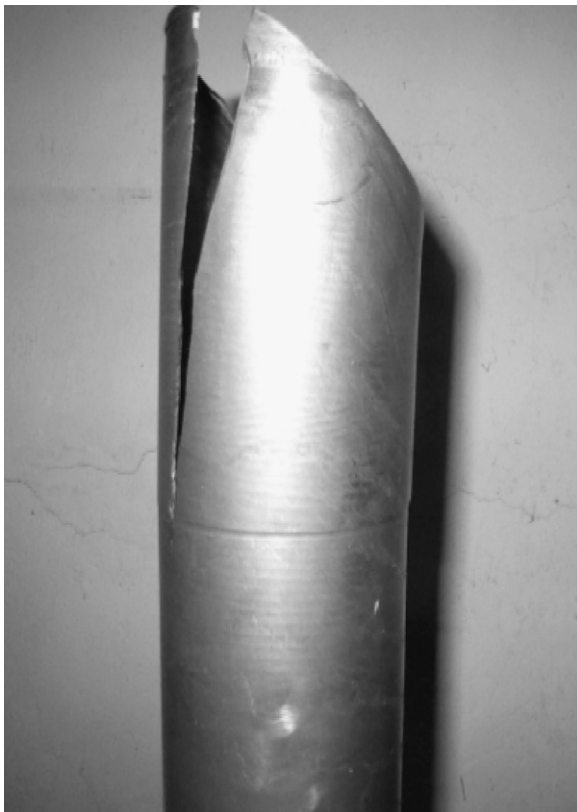
Fig. 5 – A flow-formed tube with crack-type quality problem.
