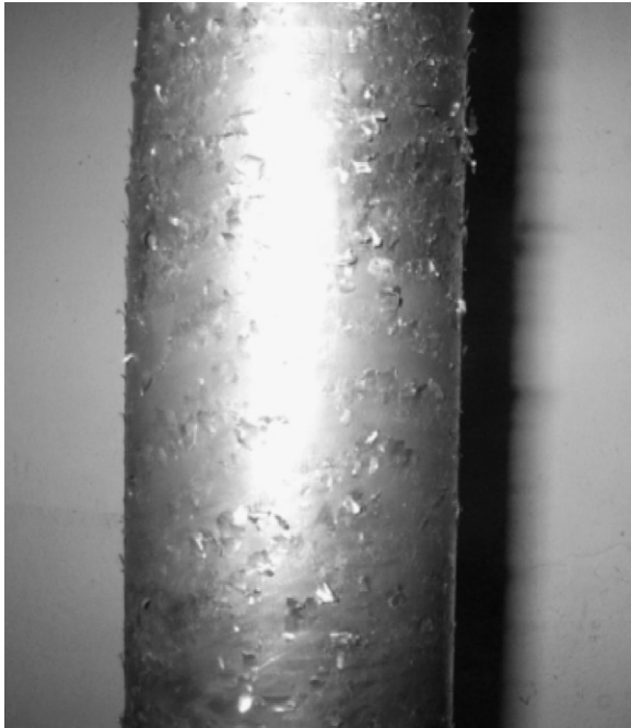
Fig. 4 – A flow-formed tube with fish scale-type quality problem.
