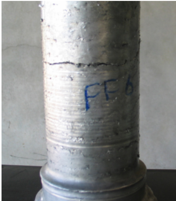
Fig. 2 – A flow-formed tube with premature burst-type quality problem.
