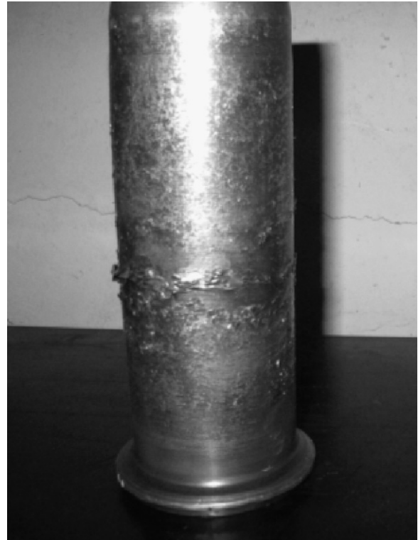
Fig. 3 – A flow-formed tube annealed for 1 h showing initial stage of fish scale.
