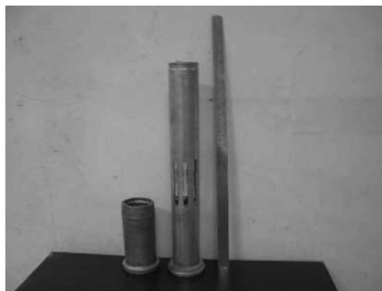
FIGURE 2.—Flow-formed AA6061 tube.
