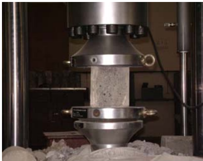
Figure 4. Compressive strength test of cube
