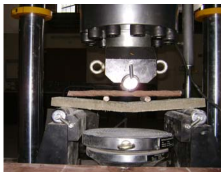
Figure 6. Flexural strength test setup
