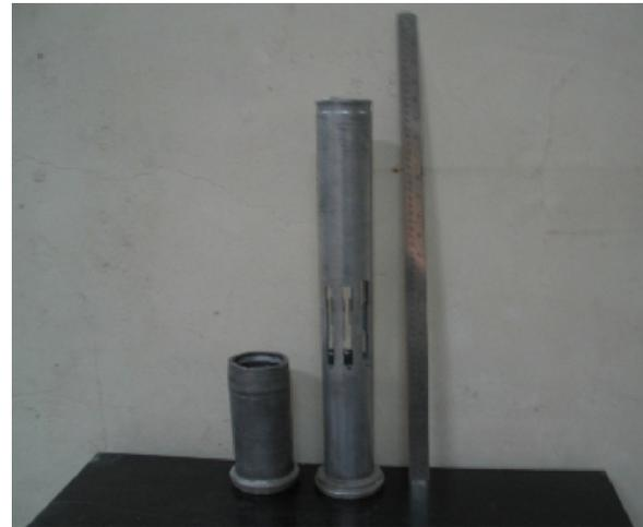
Fig. 2 – Flow-formed AA6061 tube sample.
