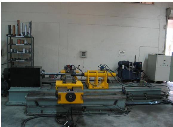
Fig. 1 – Flow-forming machine with single roller arrangement.
