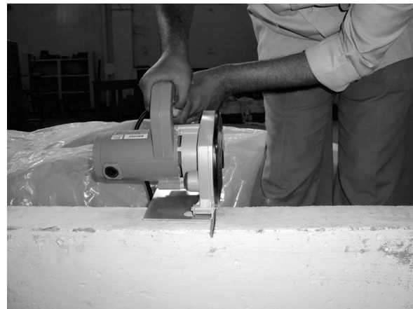
Fig. 2 Notch making in a beam using concrete cutter
