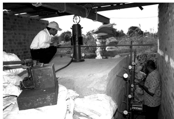
Fig. 2. Experimental setup for load testing on geotextile-reinforced (Fibertex G-100) model wall
