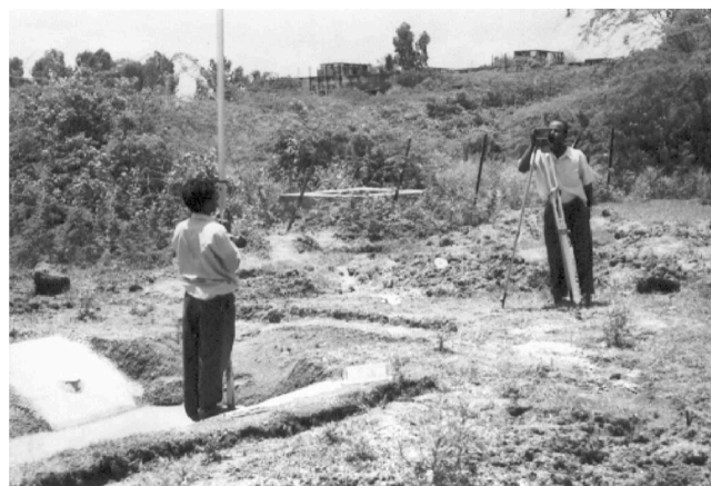
Fig. 2. Heave measurements on slopes of trapezoidal trench
