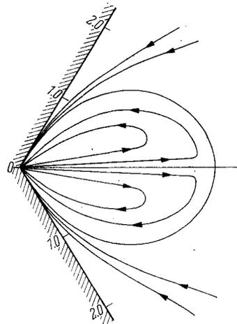
Fig. 10. Flow pattern when  $K = +1.0$  with the sink:
