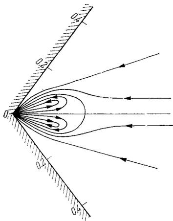
Fig. 9. Flow pattern when  $K = 0$  (Newtonian liquid) with the sink:
