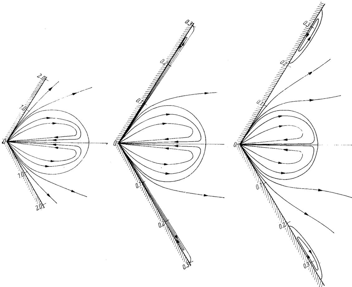
Fig. 1. Flow pattern when  $K = -1.0$  with the source:  $S = +0.1$     Fig. 2. Flow pattern when  $K = -0.001292$  with the source:  $S = +0.1$     Fig. 3. Flow pattern when  $K = -0.001$  with the source:  $S = +0.1$
