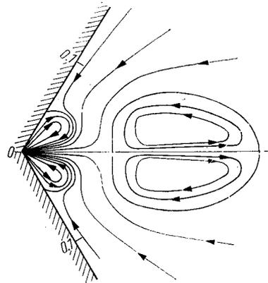
Fig. 8. Flow pattern when  $K = -0.0001$  with the sink:
