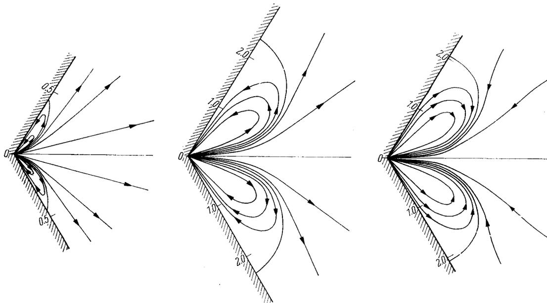
Fig. 4. Flow pattern when  $K=0$  (Newtonian liquid) with the source:  $S = +0.1$     Fig. 5. Flow pattern when  $K = +1.0$  with the source:  $S = +0.1$     Fig. 6. Flow pattern when  $K = 1.0$  with the sink:  $S = -0.1$
