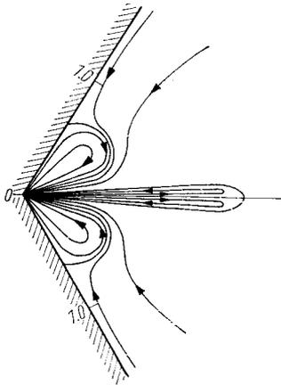
Fig. 7. Flow pattern when  $K = -0.0001933$  with the sink:
