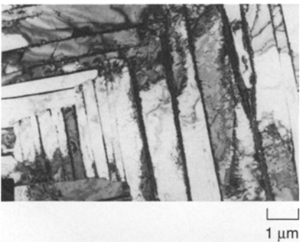
Figure 8. A TEM of the specimen deformed at 1,025°C and a strain rate of 10 s -1 .
