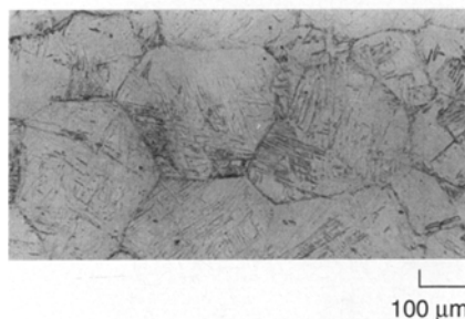
Figure 7. The microstructure of a specimen deformed at 1,025°C and a strain rate of 10 s -1 .
