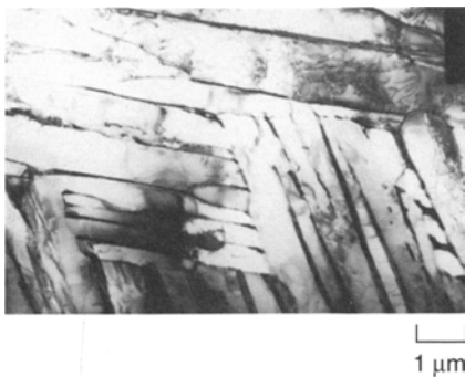
Figure 5. A TEM of a specimen deformed at 1,025°C and a strain rate of 0.001 s -1 .
