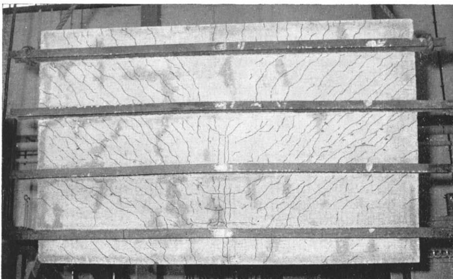
Fig. 15. Crack pattern of Model BII after failure.
