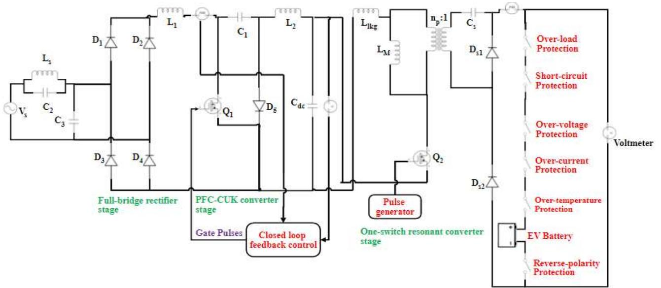
Fig. 1. Proposed PFC-CUK fed PWM resonant one-switch converter with BMS for E-bike charging.
