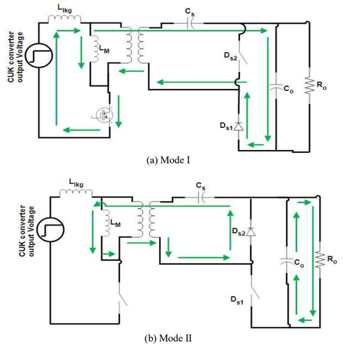
Fig. 3. One-switch resonant converter modes of operation
