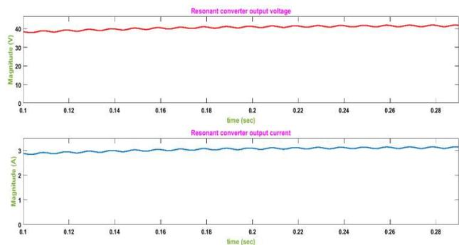
Fig. 7. Resonant converter output voltage & output current
