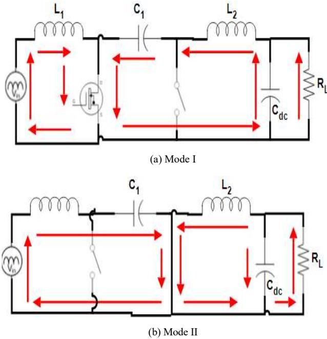
Fig. 2. PFC-CUK converter modes of operation
