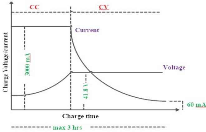
Fig. 4. CV-CC EV battery charging modes
