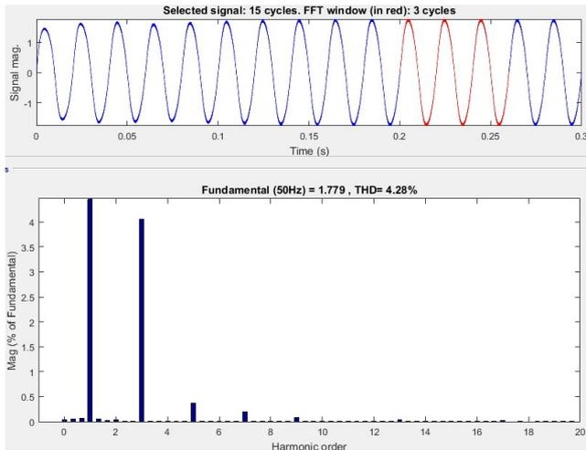
Fig. 5. FFT analysis of source current
