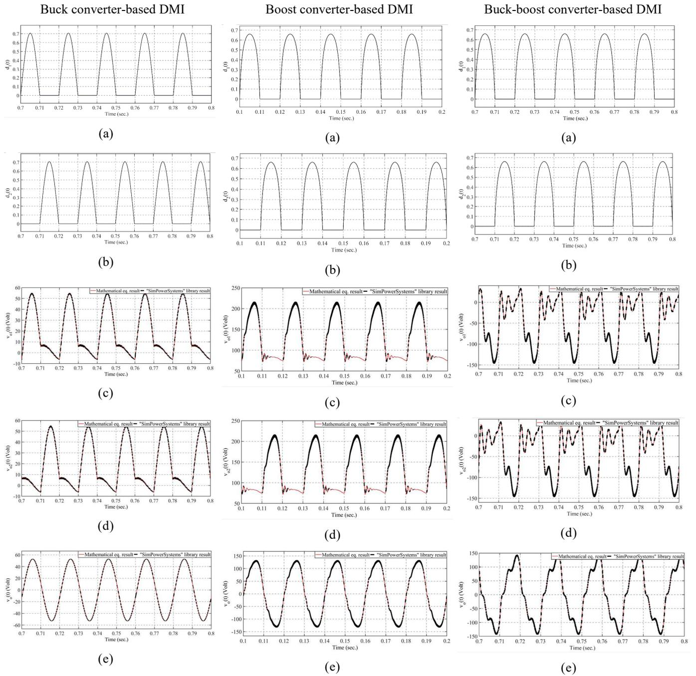
Fig. 5 Simulation results for (a) first module duty cycle, (b) second module duty cycle, (c) first module output voltage, (d) second module output voltage, (e) load voltage for buck converter, boost converter, and buck-boost converter based DMI using DMS
