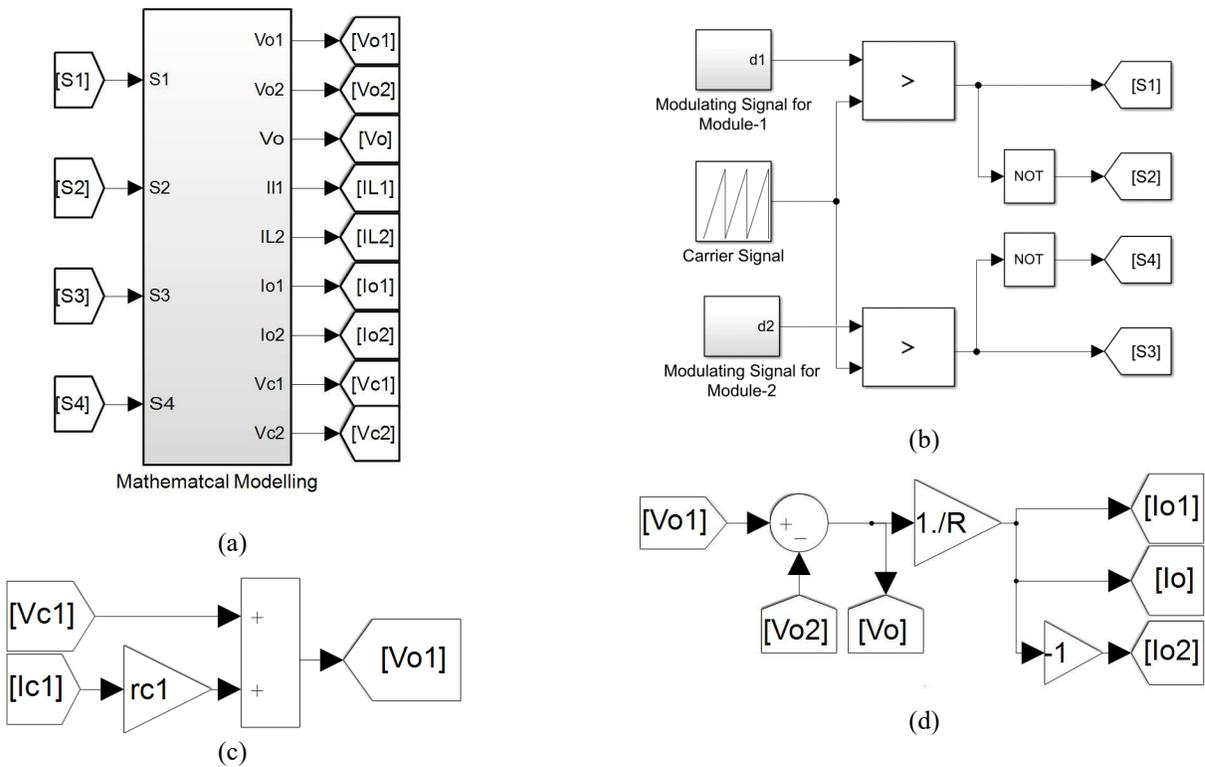
Fig. 2 Generalized (a) subsystem of DMI, (b) generation of duty cycle, (c) generation of module voltage, (d) generation of load voltage
