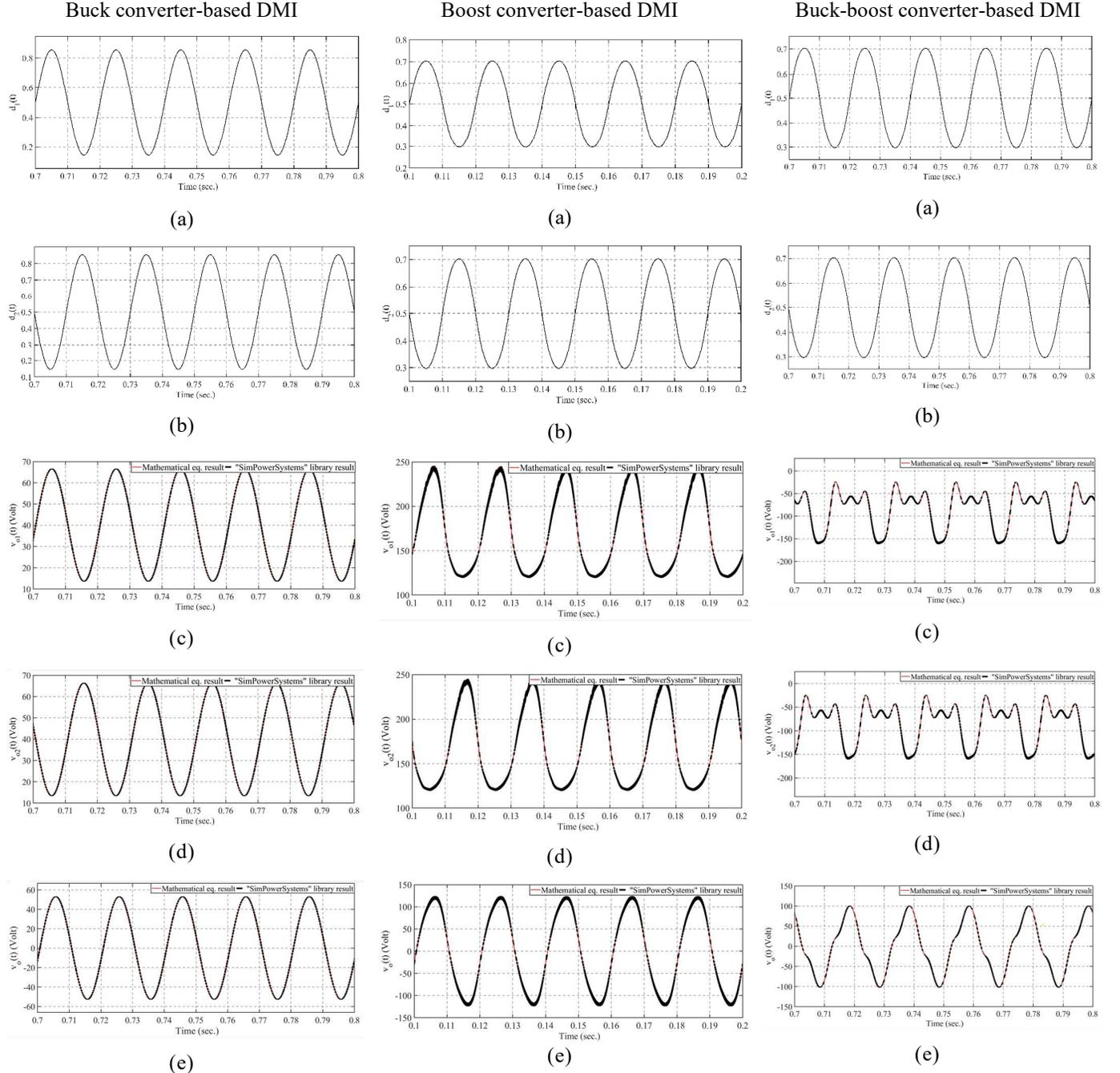
Fig. 4 Simulation results for (a) first module duty cycle, (b) second module duty cycle, (c) first module output voltage, (d) second module output voltage, (e) load voltage for buck converter, boost converter, and buck-boost converter based DMI using CMS
