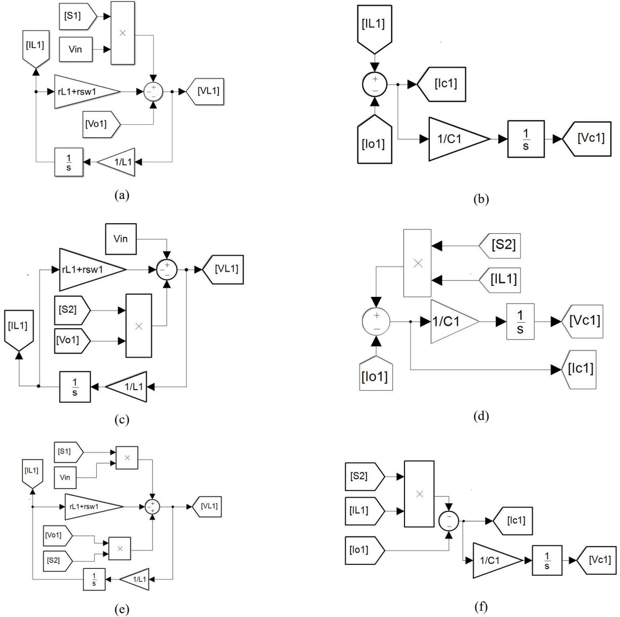
Fig. 3 Mathematical model based on (a)-(b) eq. (4)-(5) for buck converter, (c)-(d) eq. (6)-(7) for boost converter, (e)-(f) eq. (8)-(9) for buck-boost converter-based DMIs
