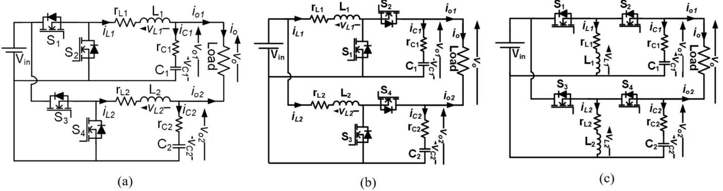
Fig. 1 (a) Buck, (b) boost and (c) buck-boost DC-DC converter-based DMI
