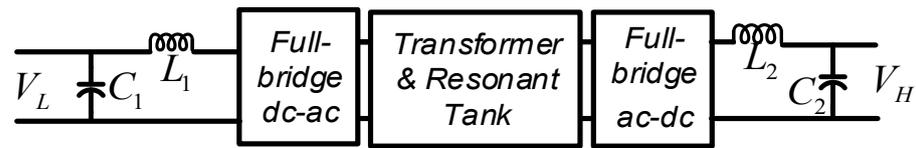
Figure 20. The common structure of DAB.
