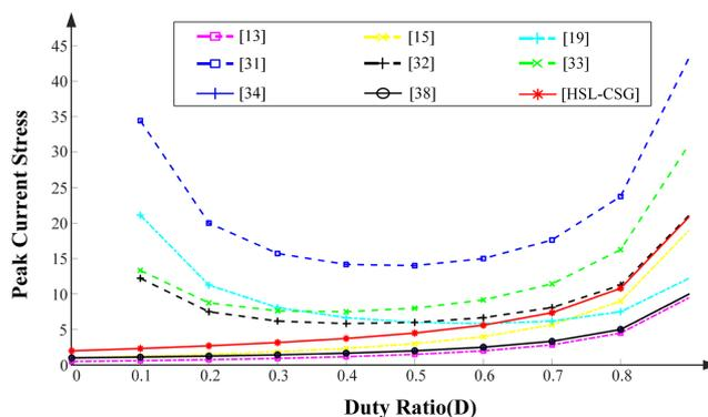
FIGURE 11 Peak current stress versus duty ratio of switches
