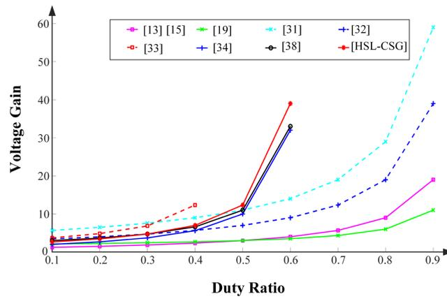
FIGURE 9 Voltage gain comparison
