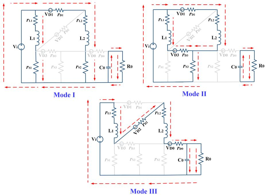
FIGURE 8 Modes of operation with parasitic parameters
