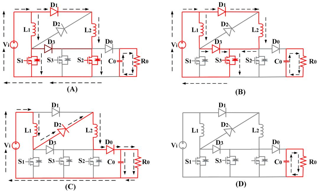
FIGURE 3 CCM and DCM operation (A) S<sub>1</sub>, S<sub>2</sub> ON for Mode I; (B) S<sub>3</sub> is ON for Mode II; (C) S<sub>1</sub>, S<sub>2</sub>, S<sub>3</sub> are OFF for Mode III; (D) equivalent circuit of Mode IV (for DCM only)
