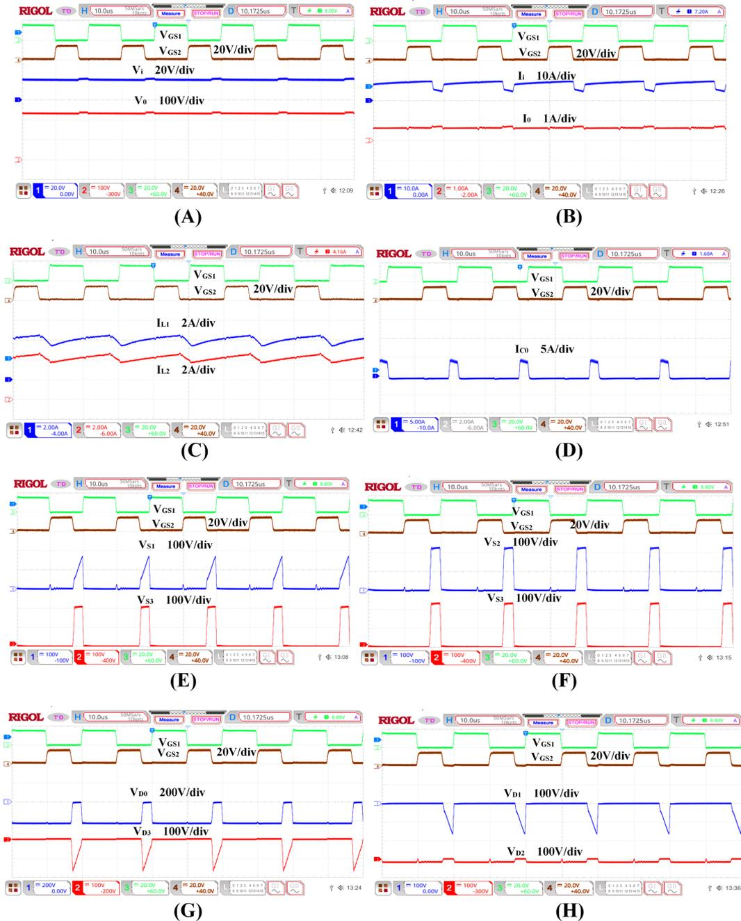
FIGURE 13 Experimental results. (A) Input and output voltages ( $V_i$  and  $V_o$ ); (B) input and output currents ( $i_i$  and  $i_o$ ); (C) inductor currents ( $i_{L1}$  and  $i_{L2}$ ); (D) capacitor current ( $i_{C0}$ ); (E) switch voltages ( $V_{S1}$  and  $V_{S3}$ ); (F) switch voltages ( $V_{S2}$  and  $V_{S3}$ ); (G) diode voltages ( $V_{D0}$  and  $V_{D3}$ ); (H) diode voltages ( $V_{D1}$  and  $V_{D2}$ )
