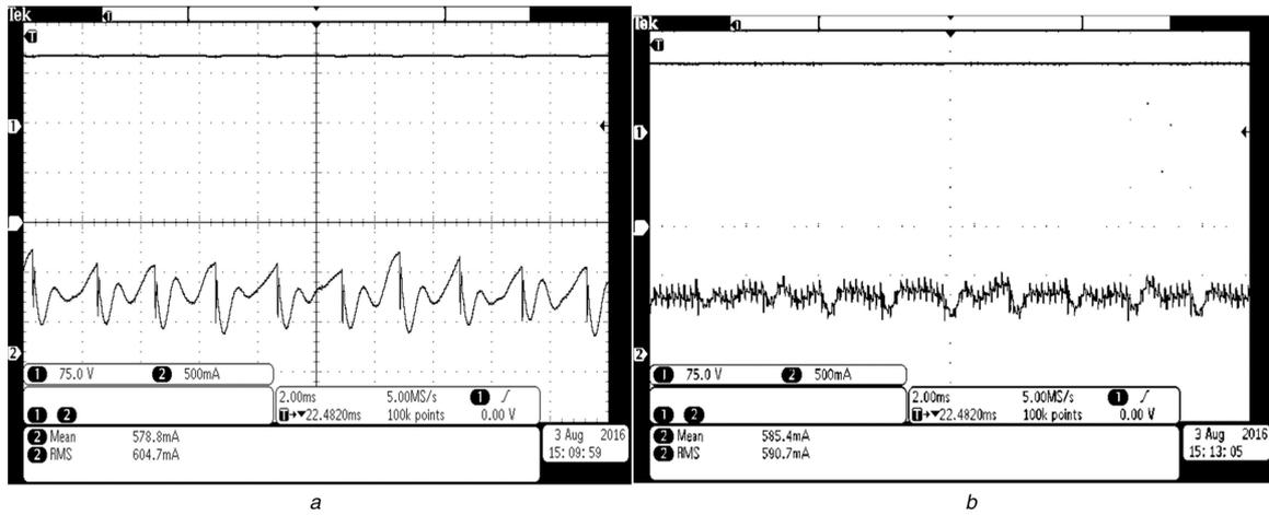
Fig. 9 DC-link current with ripple (scaling factor of 0.54)
