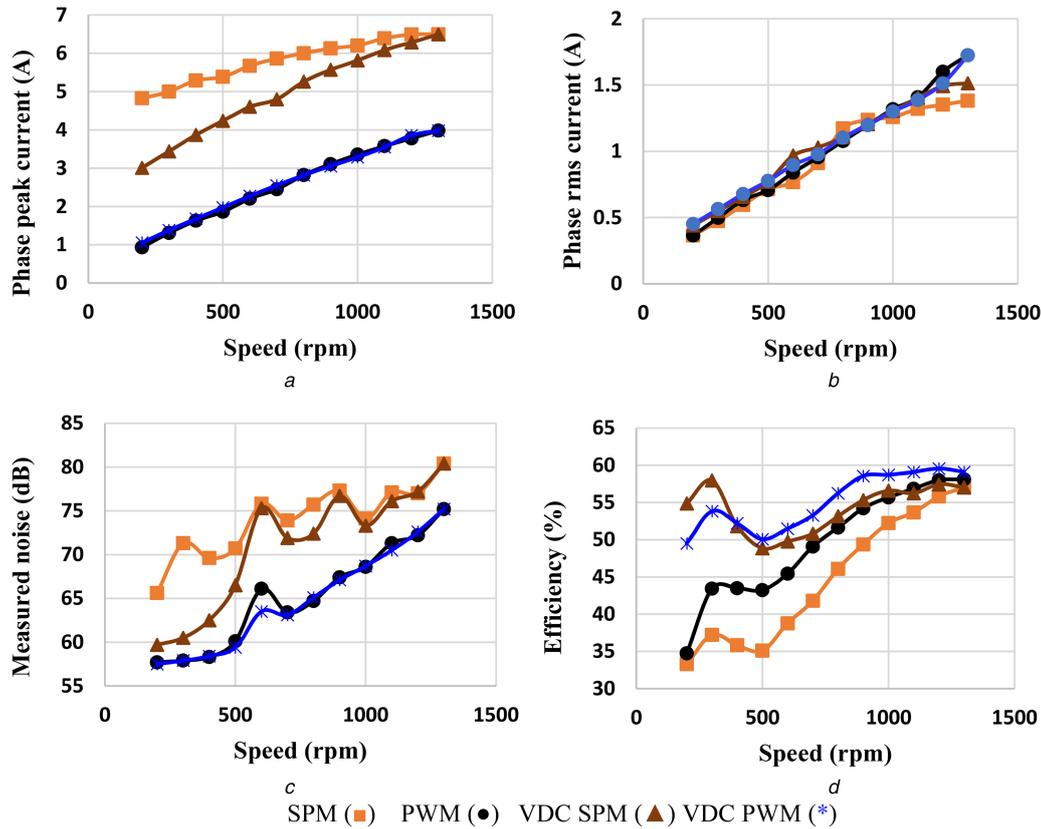
**Fig. 5** Characteristics of various performance parameters versus speed for all control schemes
