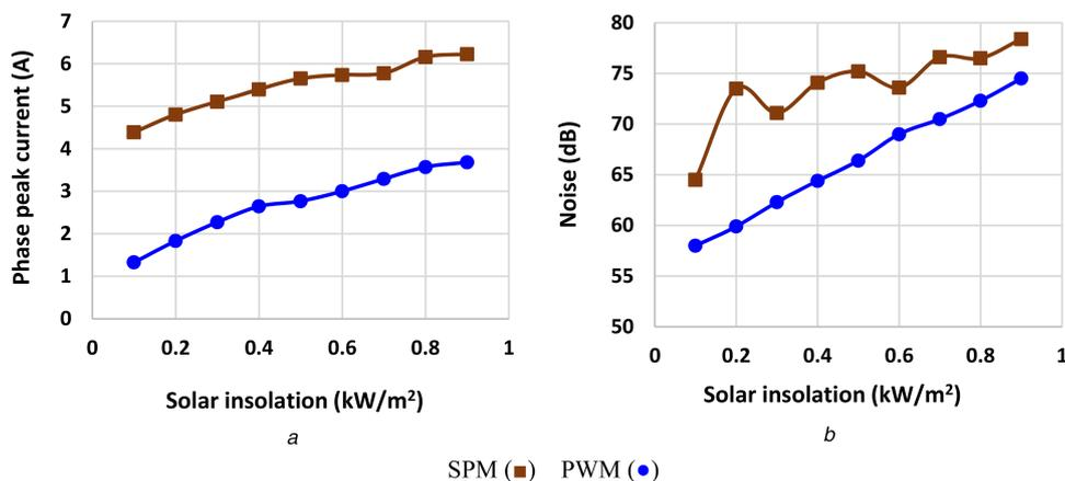
**Fig. 8** Performance characteristics of direct PV-fed SRM-WPS
