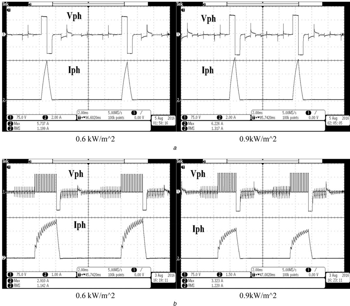
**Fig. 7** Experimentally measured phase voltage and current
