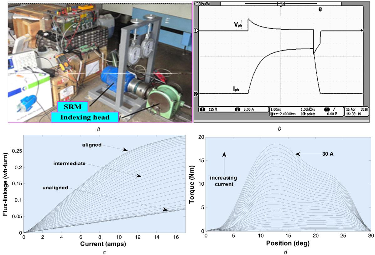
**Fig. 2** Experimentally obtained flux-linkage and static torque characteristics
