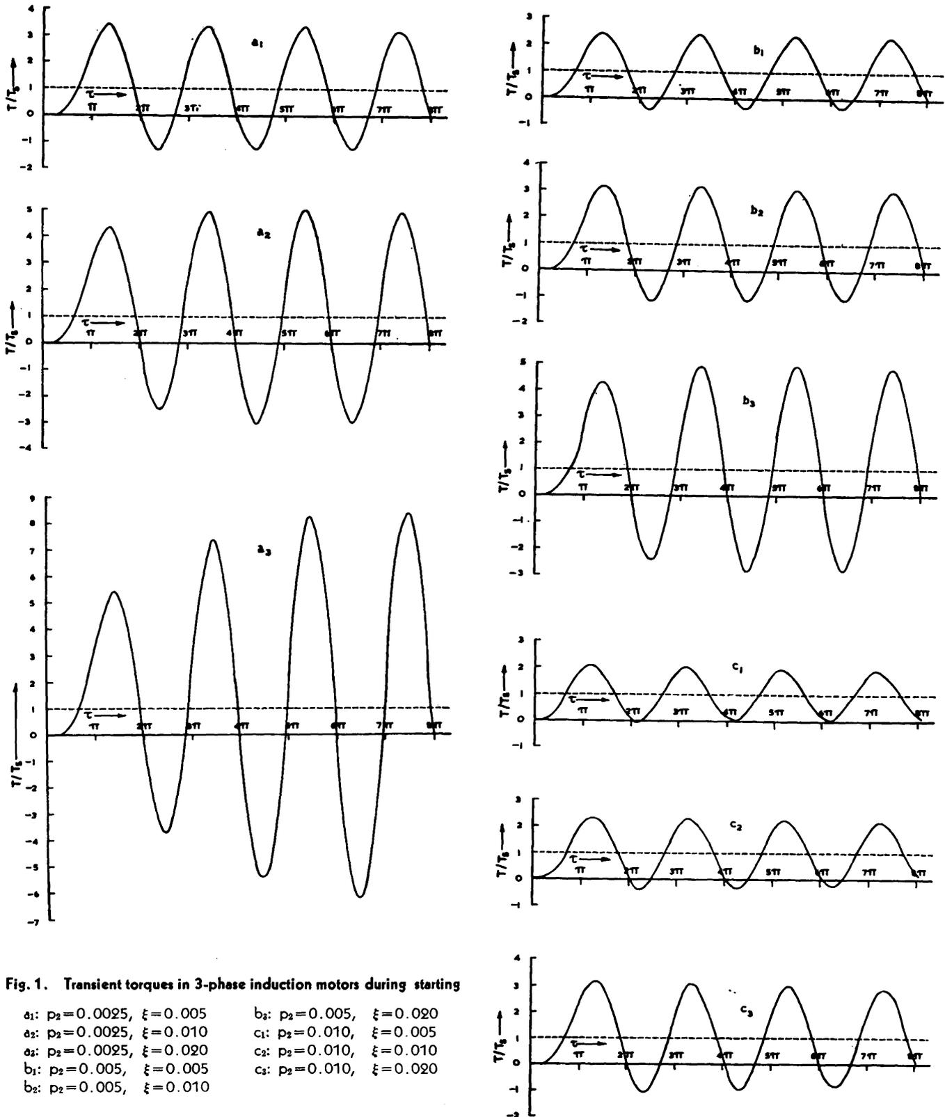
Fig. 1. Transient torques in 3-phase induction motors during starting
