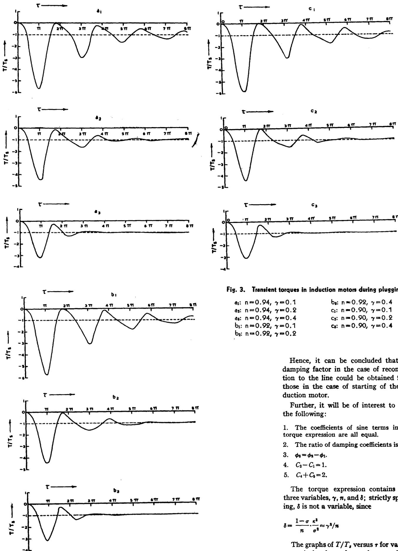
Fig. 3. Transient torques in induction motors during plugging
