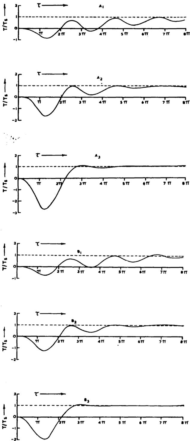
Fig. 2. Transient torques in 3-phase induction motors during reconnection to line
