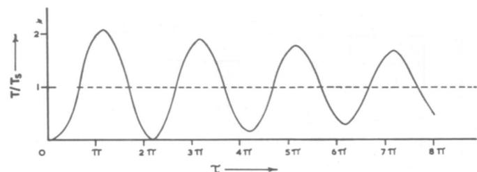
**Fig. 5. Theoretical curve of the transient starting torque for the motor under test**
