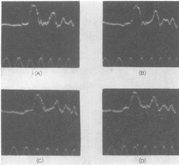
**Fig. 4. Transient starting torques obtained by experiment**
