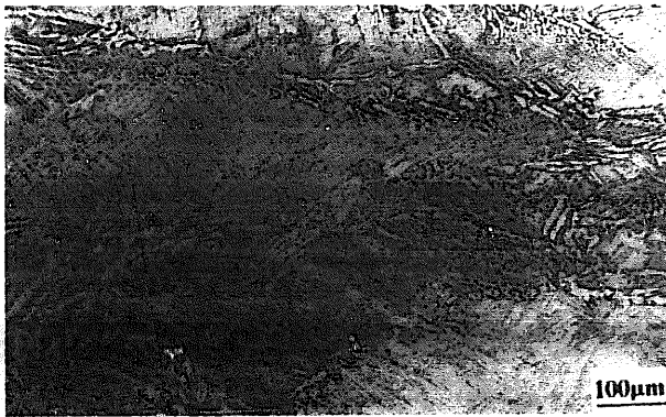
Fig. 6. Microstructure of a specimen deformed at 975°C and 0.001 s -1 , revealing sluggish coarsening of \alpha laths, particularly at grain interiors.
