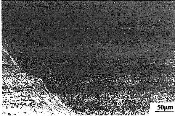
Fig. 5. Microstructure of a specimen deformed at 925°C and 0.001 s -1 showing the tendency of the breaking-up of the acicular \alpha .
