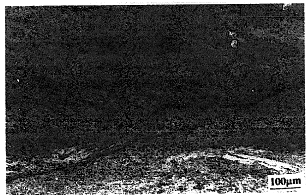
Fig. 9. Microstructure of a specimen deformed at 875°C and 10 s -1 exhibiting a crack path oriented at about 45° to the compression axis, along with an adiabatic shear-band zone.
