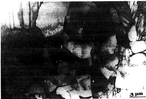
Fig. 7. Transmission electron micrograph of a specimen deformed at 975°C and 0.001 s -1 , exhibiting a mixture of sub-grains and \alpha laths.
